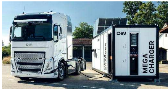
E-LKW: High-Power-Charger (HPC)
